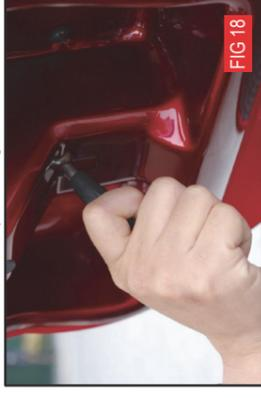
The handlebar lock is operated by a black lever positioned handlebar (see Fig 18). To release the handlebar from a locked position pull the black lever upwards, the handlebar will now move freely, but under mild tension.
