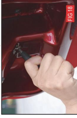
The handlebar lock is operated by a black lever positioned handlebar (see Fig 18). To release the handlebar from a locked position pull the black lever upwards, the handlebar will now move freely, but under mild tension.
