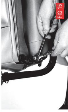
**⚠ Warning:** Both stop bolts must be positioned in the same position for the backrest to be fully supported, failure to observe this warning may distort the backrest frame.
