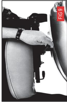
**Warning:** When driving, the seat should be locked in the straight ahead position.
