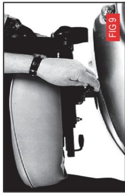
**Warning:** When driving, the seat should be locked in the straight ahead position.
