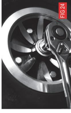
3. With the aid of two 13mm spanners (not supplied) deflate tyre as necessary before remove the 8mm nuts and bolts from the wheel rim and centre hub. (Have you deflated the tyre?)
