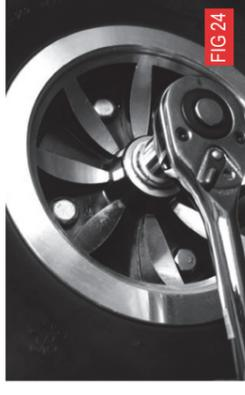
3. With the aid of two 13mm spanners (not supplied) deflate tyre as necessary before remove the 8mm nuts and bolts from the wheel rim and centre hub. (Have you deflated the tyre?)
